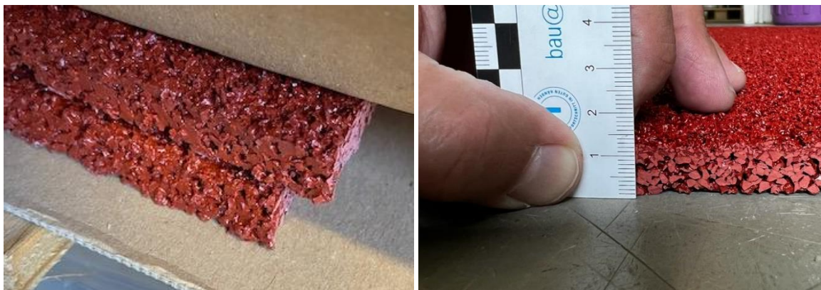
Fig. 1, 2: Synthetic surface product " CONIPUR EPDM/SP 11+3mm ", sample received by OFI on 03.05.2022 (fig. 1, left) and 10.05.2023 (fig. 2, right)
